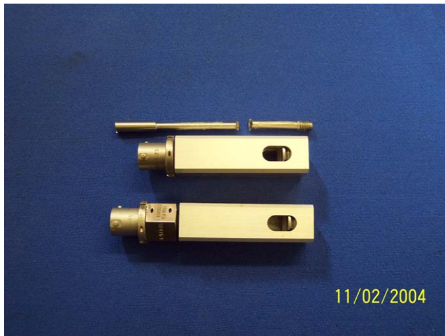
SL1056-6 Mini Cutter with single PC-23 Initiator SL1056-6 Mini Cutter with single PC 154 (Booster) Initiator
